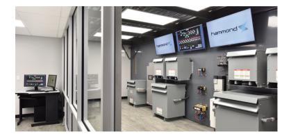
The HPS Power Quality Lab allows customers to experience real time testing of line side HPS power quality products such as transformers, line reactors, active harmonic filters and passive harmonic filters as well as load side products such as load reactors, sinewave filters and different types of dV/dT filters with various cable lengths. The power quality products can run at full load using either 10HP, 25HP and 100HP VFD systems and associated motor/load.
