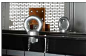
Lifting eyes for core & coil assembly
