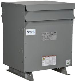
The use of K-factor distribution transformers has become a popular means of supplying power for non-linear loads such as electronic ballasts, drives, personal computers, telecommunications equipment, broadcasting equipment and other similar power electronics. These non-linear loads generate harmonic currents which can substantially increase transformer losses. Our K-rated transformers have been specifically designed to prevent failure due to overheating.
