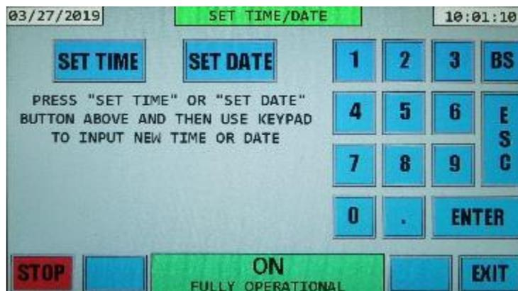
This display has the 2 buttons "SET TIME" and "SET DATE", along with a keypad. Press the "SET" function desired, and use the keypad to enter the correct time or date. When done changing the time and/or date, press the EXIT button to exit back to the main menu.
