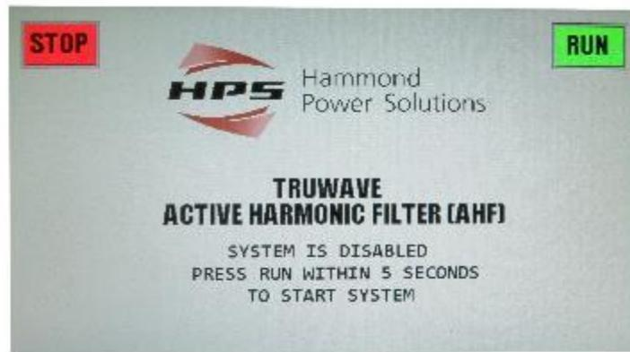
Do not press RUN when powering on the unit for the first time. After 5 seconds the “OPERATING STATUS” display page will appear. Pressing the STOP button when the splash screen is displayed will immediately send you to the “OPERATING STATUS” display instead of waiting the 5 seconds.
