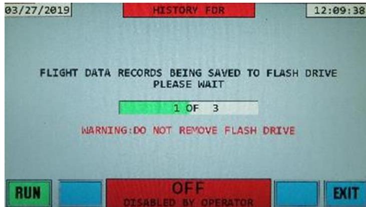
**Note:** Do not remove the flash drive while the FDRs are being saved, as this may cause the file and or the flash drive to be corrupted. If once you start saving FDRs you decide you don't want to save all of the selected FDRs, simply press the EXIT button. After the current FDR being saved completes, no additional FDRs will be saved.
