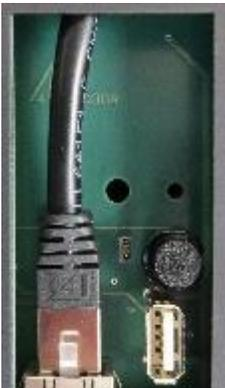
Also in this compartment is a Cat-5 cable plugged into a RJ45 connector. This is the Ethernet connection that gets routed to the top access point of the HMI enclosure. One can remove this cable from this connector and plug another Cat-5 cable into the RJ45 connector, and go to a computer or network with the added cable to look at data or parameters over the Ethernet connection. This allows access to the Ethernet
