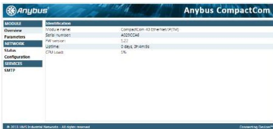
Click on Status under NETWORK to see more detailed network information. Click on Configuration under NETWORK to set a Static IP Address.
