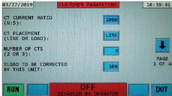
3. Note that the parameter values are now inside blue rectangles surrounded by grey borders. This indicates that these are now buttons that can be to change the parameter desired. In the following example we will modify the CT PLACEMENT parameter from the value LINE to the value LOAD.
