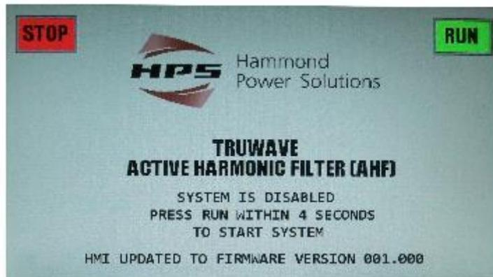
As an additional verification you can open the CONFIGURATION PARAMETERS DISPLAY as described in section 5.6.3 and verify that the HMI Software version matches the version number of the file. In our example we updated the HMI firmware with HMI01000.BIN, and in the CONFIGURATION PARAMETERS display the HMI Software Version is 001.000. See picture below.
