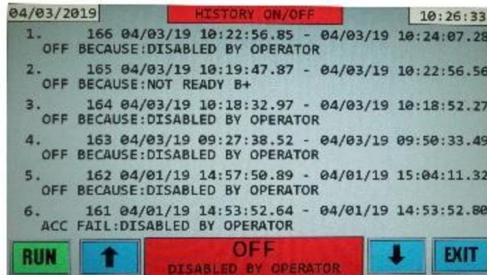
The display contains 2 lines of data for each shutdown event. The events are displayed from newest to oldest. Using the arrow buttons on the bottom of the display it’s possible to navigate the database to view even older events, up to 480 events. The first number in each row with a period after it, is the event number with number 1 being the latest event. The second number in each row is the internal database
