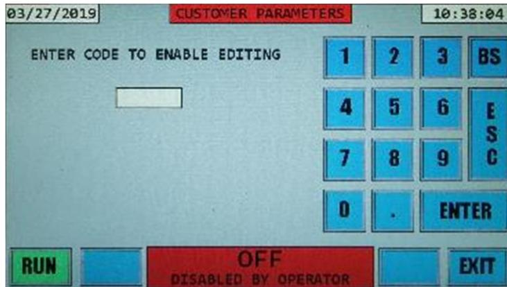
2. Using the keypad, enter the code "1076" and press Enter. Use the backspace button "BS" to delete an incorrectly entered character. The following screen should open.
