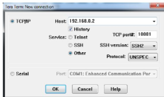
Note that the IP Address is 192.168.0.2. Tera Term will not connect if you include the leading zeros in the IP Address. Also, note that this is the IP Address that we set in the HMI in step 4. The TCP port is 10001. If you click OK, and then press the Enter key, you should see > prompt symbols. Type s and press Enter. You should see the system status information. This verifies that the HMI is communicating with your computer.
