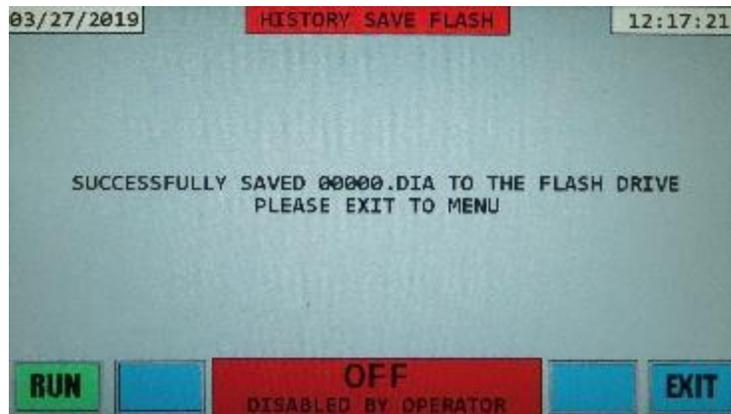
The file will be named with the same number as the DSP board serial number and have the extension .DIA for diagnostic.
