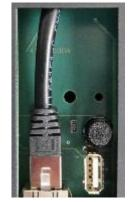
top screw, then just loosen the bottom screw so that you can swing the front cover open, exposing the components as shown in the picture to the right. The USB connector can be used to plug in a flash drive. The HMI via the LCD display can be instructed to download various stored history data to the drive (see section 5.8 for additional details).
