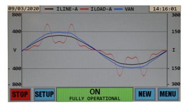
The three multicolored bars to the left of the waveform titles show what color is used to display each waveform. There are two separate grids, one for the voltages on the left with the letter V representing 0 volts, and one for the currents on the right with the letter I representing 0 amps. If only voltages are displayed, the grid on the right would not be displayed. Likewise, if only currents are displayed, the grid on the left would not be displayed.
