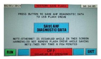
First make sure that a USB flash drive is inserted into the USB port on the front panel. The flash drive USB port is located under the protective cover to the right of the LCD screen on the front panel of the HMI. Refer to section 3.5.6 on opening the cover and locating the USB port.
