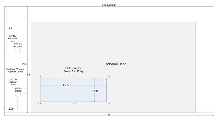
Figure 3.8: 400Amp AHF Type 1 Cabinet Top Wire Entry
