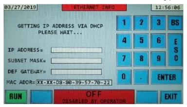
The system will now determine an IP address, Subnet Mask, and Default Gateway Address via DHCP, and display the new information on the screen. The option to go back to a static IP address is still available via the CHANGE TO A STATIC IP ADDRESS button which now appears at the top. See the following picture.
