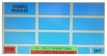
After selecting "DISABLE MODULES", you'll be brought to a screen where you can "DISABLE" or "ENABLE" Module 1 or Module 2. The image below currently shows Module 1 Enabled and Module 2 Disabled. This feature can be used for testing and troubleshooting purposes.
