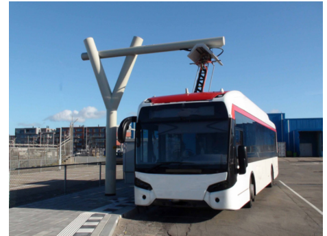
Multiple Class 3 chargers can create significant power quality issues. Proper selection of transformers can help to mitigate these issues.
